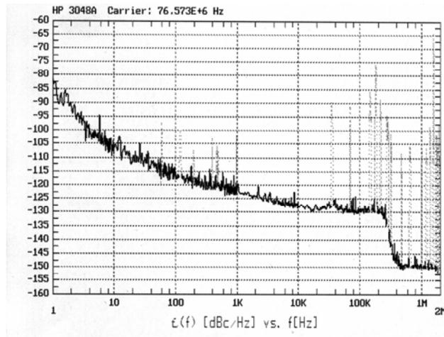
Figure 8. Typical channel phase noise from mix/multiply/DDS architecture.
