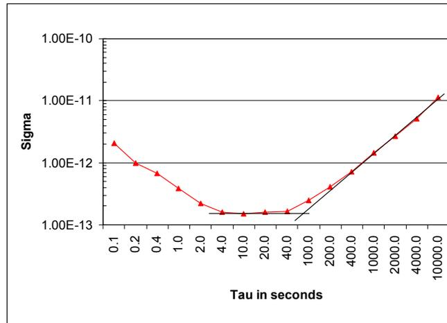
Figure 7. Allan deviation characteristic of the synthesized MTP USO.
